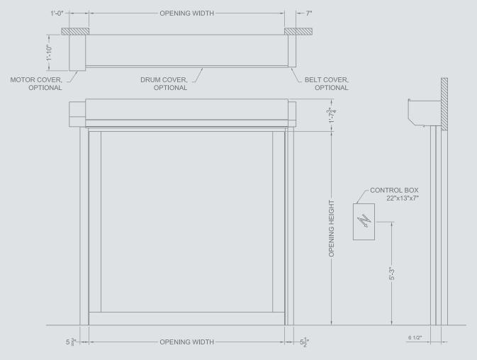
All indicated dimensions are minimum space requirements for installed door.
