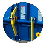
An integral safety stand works with the built-in maintenance strut to provide added safety during maintenance, servicing, and cleaning.\*
